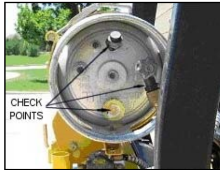
Figure 4-1. Examples of leak check points on LPG tank
