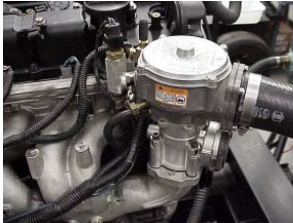
Figure 1-13. CA100 Mixer Installed with Electronic Throttle
