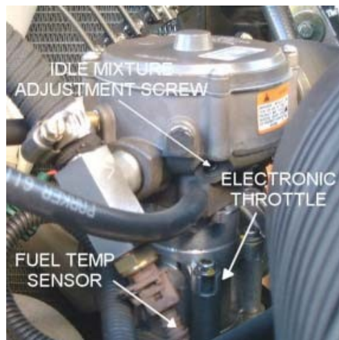
Figure 1-14. Idle Mixture Adjustment Screw (with tamper proof cap removed)
