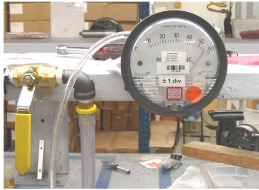
Figure 6-3. Magnehelic Gauge Connection to Hose Barb
